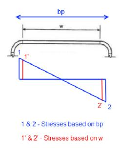
$\sigma_{\text{beg}}$ : normal stress at start point of rectangular shape – compression stress is positive  $\sigma_{\text{end}}$ : normal stress at end point of rectangular shape – compression stress is positive
