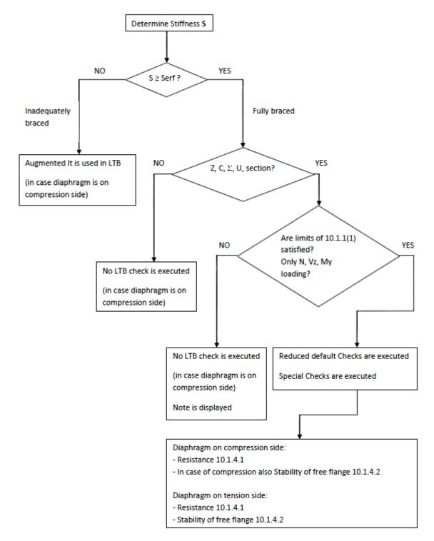
$$S = \frac{a \cdot 10^4}{K_1 + \frac{K_2}{L_s}} S_{erf} = \left( E I_w \frac{\pi^2}{L^2} + G I_t + E I_z \frac{\pi^2}{L^2} 0,25 h^2 \right) \frac{70}{h^2} I_{t,id} = I_t + vorC_\theta \frac{l^2}{\pi^2 G}$$
