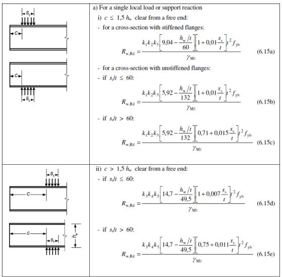
Figure 6.7a): Local loads and supports - cross-sections with a single web
