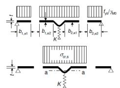
b) Step 1: Effective cross-section for  $K = \infty$  based on  $\sigma_{\rm com, Ed} = f_{\rm yb}/\gamma_{\rm M0}$
