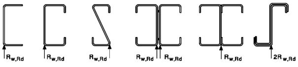
Figure 6.6: Examples of cross-sections with a single web
