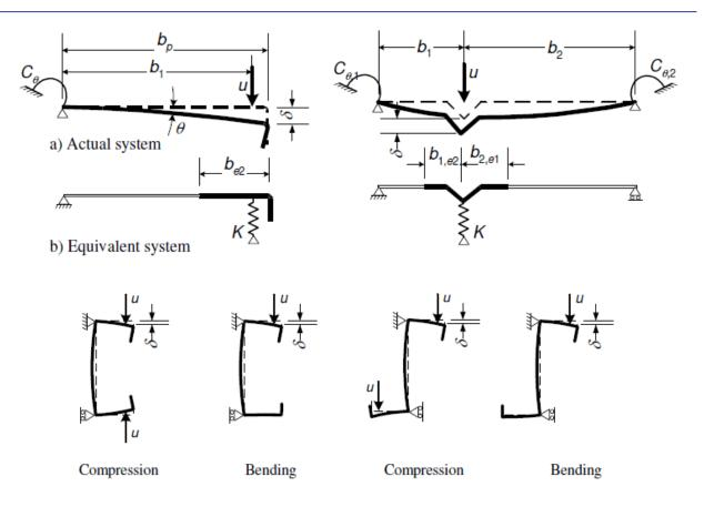
c) Calculation of  $\delta$  for C and Z sections
