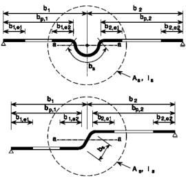
Figure 5.9: Intermediate stiffeners
