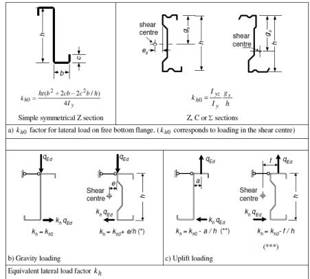
(\*) If the shear centre is at the right hand side of the load  $q_{\rm Ed}$  then the load is acting in the opposite direction.
