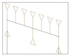
The default LTB data, defined in the buckling data dialog, are overruled by the LTB restraints. Fixed LTB restraints are defined on the top flange or on the bottom flange. The LTB lengths for the compressed flange are taken as distance between these restraints. The LTB moments factors are calculated between these restraints.
